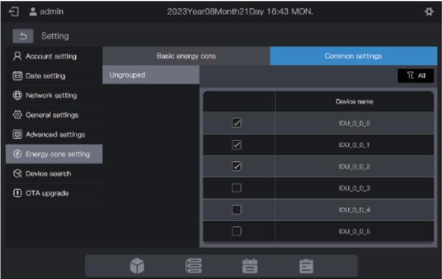
The selected devices are public devices and unselected devices are enabled devices. Click **ALL** to filter all devices, public devices, and enabled devices. As shown in the figure below, click a device to view its device type.
