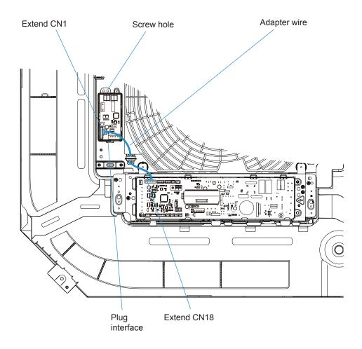
Step 3: Remove the mounting box cover from the accessory package, and fasten the cover to the base of the adaptor board as shown in the figure below. Note that the communication adaptor wire should be led out from the outgoing wire hole.
