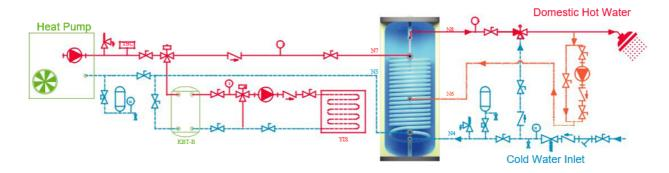
Important notice: maximum 8 bar safety valve must be installed.
