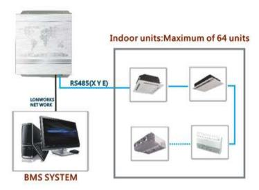
This connection method is suitable for all of the air conditioners system.
